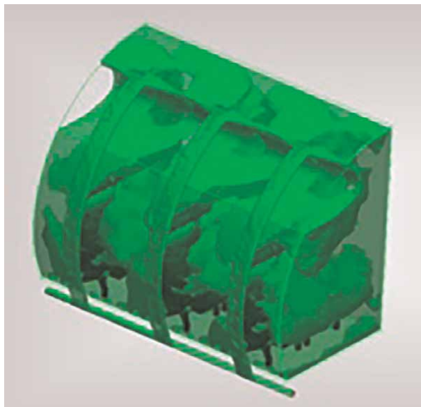
Figure 16. Iso surface are surfaces that represent points of a constant number. For example, temperature and airspeed.
