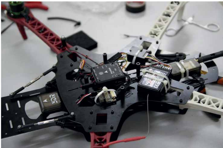
Figure 6. Assembly of GPS module and radio telemetry.
