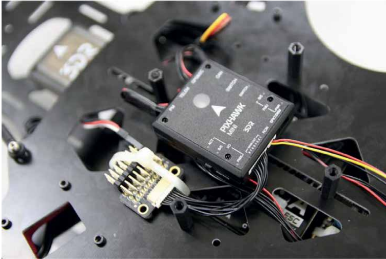
Figure 5. Pixhawk mini flight controller mounting.
