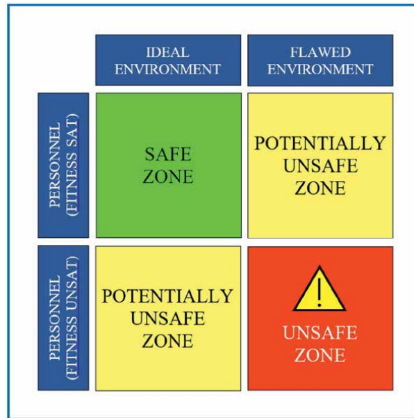
Figure 9. Safe, potentially unsafe, and unsafe zones.
