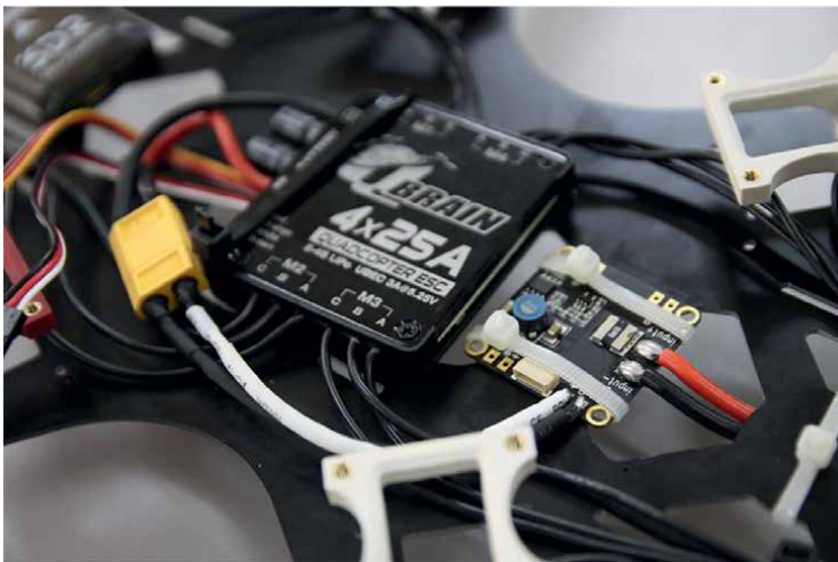
Figure 4. Mounting of the power module.
