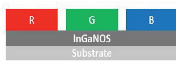
Figure 11. Schematic of InGaN LED structures grown on InGaNOS modified substrate.
