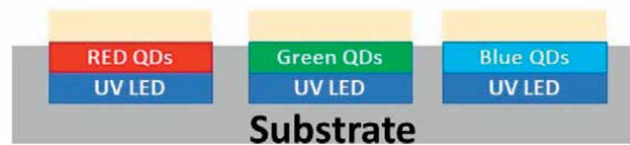
Figure 12. Schematic of UV micro-LED and QDs integration approach to realize the full-color pixel.
