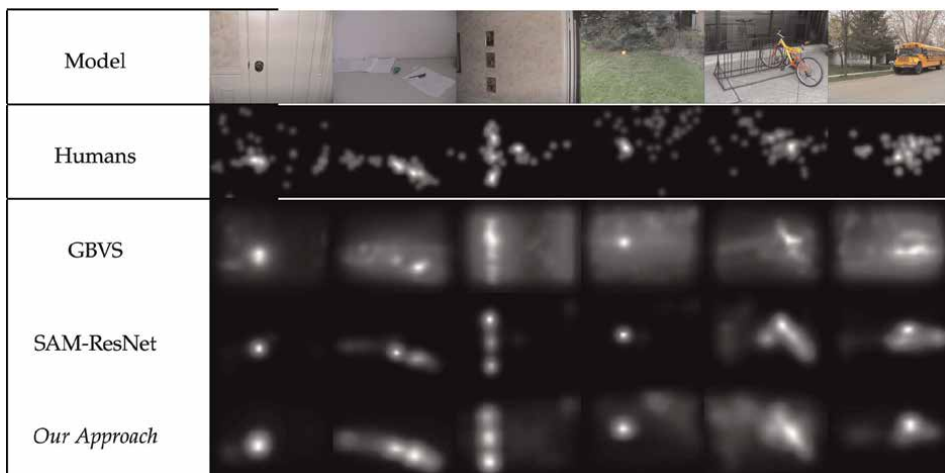
Figure 3. Qualitative results for real images (Toronto dataset). Each image is represented in a different column and each model saliency map in each row. The ground truth density map of human fixations is represented in the second row.
