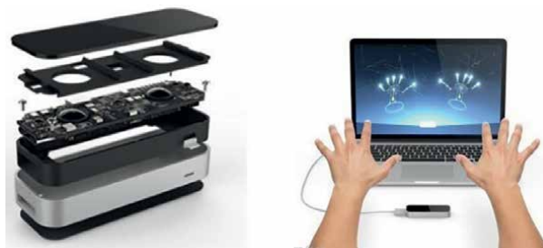
Figure 1. Leap motion controller (LMC). Source: Leap motion, 2019 https://www.leapmotion.com/ .
