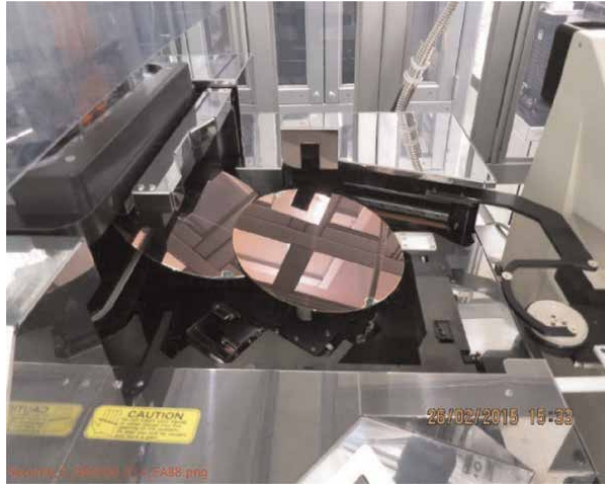
Figure 1. Wafer damage caused by positioning deviation of robot end effectors during manufacturing.
