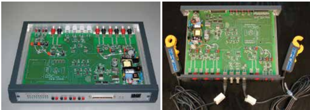
Fig. 10. Layout of the conditioning system, SAC-2.
