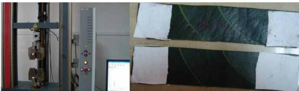
Fig. 10. The tension test of plant leaf
