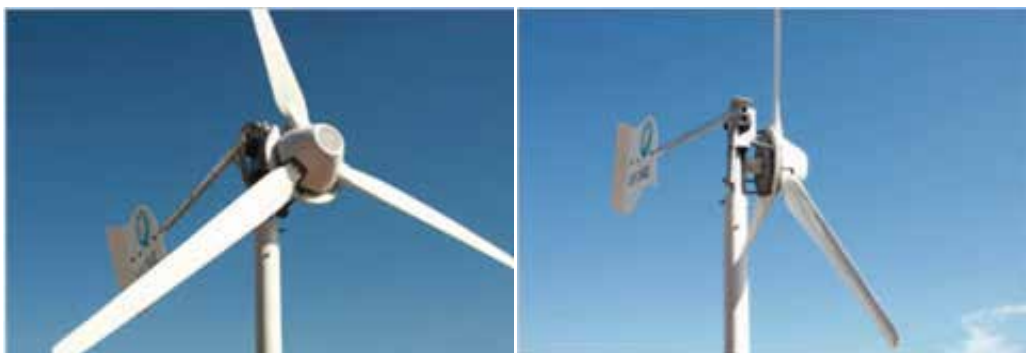
Fig. 9. Furling mechanism operating in a commercial wind turbine rated at 1.4kW. (a) Normal (unfurled) operation. (b) Furled turbine.
