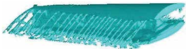
(b) Blade topology optimization result
