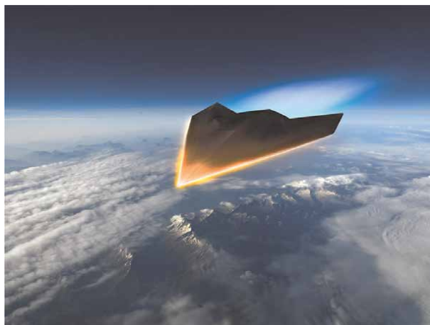
Figure 1. Hypersonic glide vehicle, leading edges experiencing high friction and heat loading [1].
