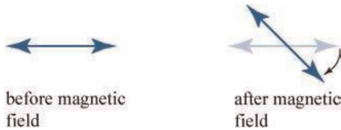
Figure 3. Rotation of a light ray by a magnetic field [4].
