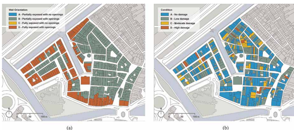
Figure 7. Spatial distribution of (a) wall orientation and (b) building condition parameters.
