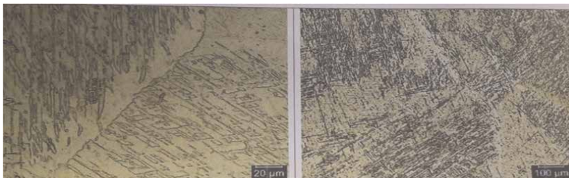
Figure 20. The microstructure of the heat affected area with two magnifications for 80 amps.
