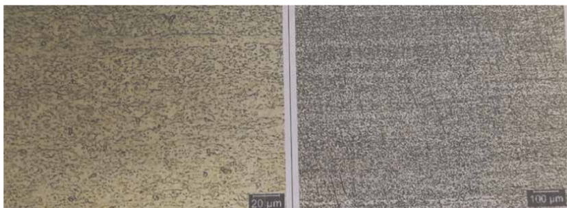
Figure 19. Basic metal microstructure with two magnifications for 80 amps.
