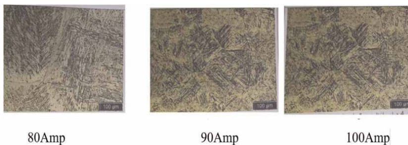
Figure 23. Heat affected area microstructure in three different samples: A(80 Amp), B(90 Amp), C(100 Amp).
