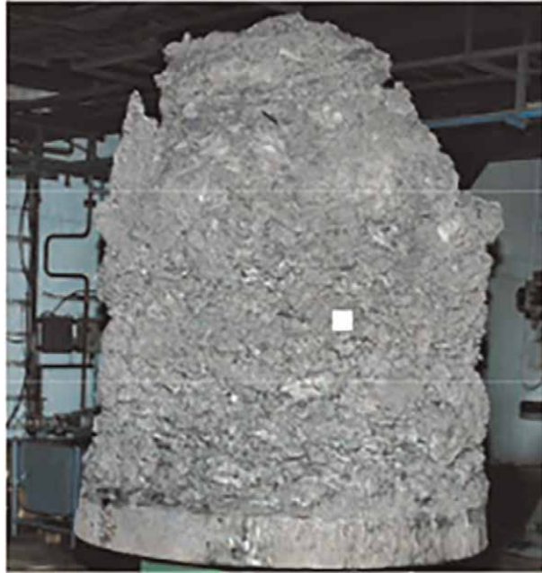
Figure 3. A 3 MT titanium sponge cake produced at DMRL titanium experimental facility by combined process technology.
