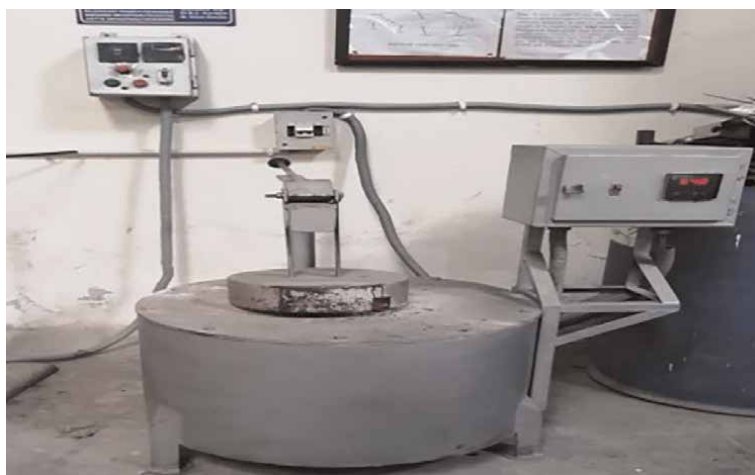
Figure 4. Electric furnace used for HMMC development.
