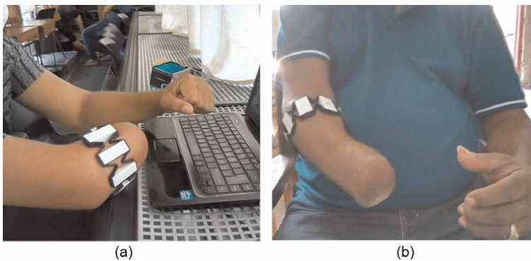
Figure 4. (a) Amputee patient in front of the computer with a graphic signal to perform the movements. (b) MYO device arrangement.
