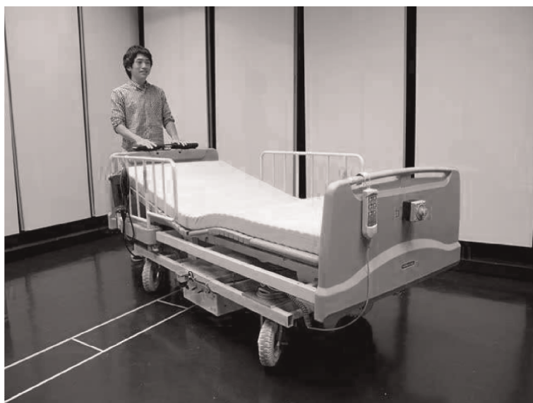
Figure 7. Power-assisted nursing care bed developed by the Authors can be moved in Omnidirectional. The traveling cart, which is add-on to a commercially available care bed, can be easily moved back and forth, left and right, and swiveled by a single person by lightly applying force to the operating handle.
