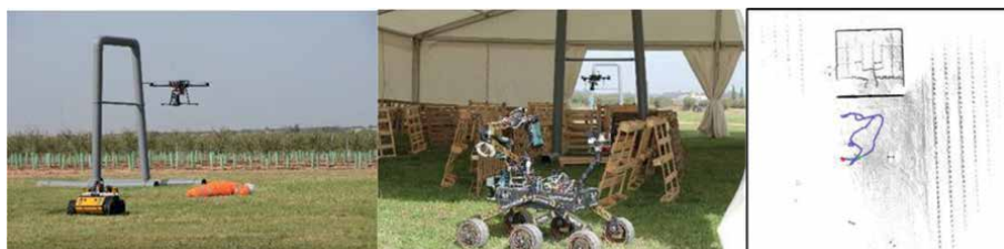
Figure 6. (left) the UAV and UGV from team LARICS in action, reaching the outdoor missing worker. (Centre) the rover UGV and the UAV from team raptors looking for the indoor missing worker. (right) top view of a 3D map of the competition area by team LARICS. The trajectory followed by the robot is shown in blue.
