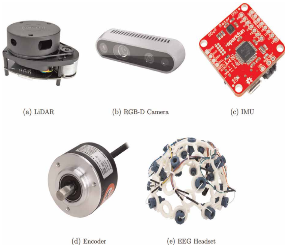
Figure 3. Various electronic sensors: (a) LiDAR, (b) RGB-D camera, (c) IMU (d) encoder and (e) EEG headset.
