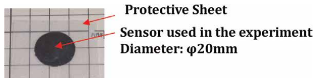
Figure 8. An experimental sensor with a diameter of 20 mm.
