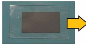
Figure 15. Sample photograph of a stretch sensor (using carbon grease electrode): Measure the change in conductivity while increasing the stretch by 0.5 cm in the right direction of this sample.
