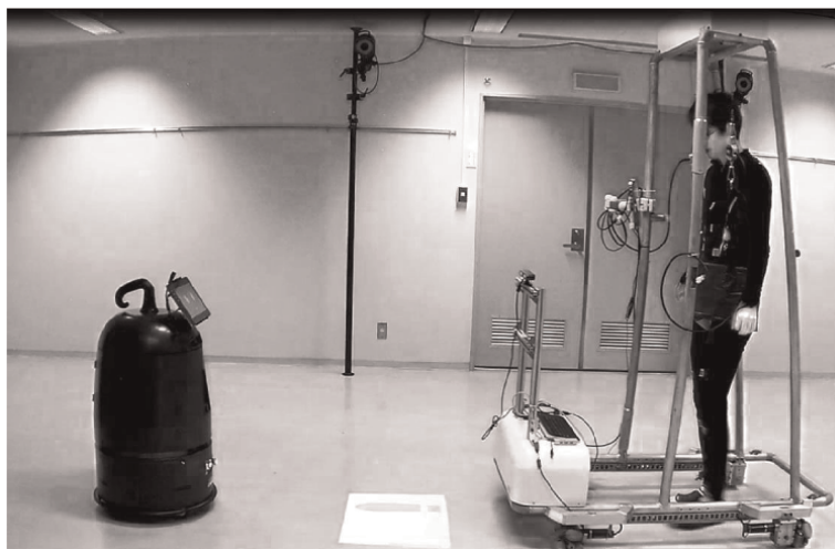
Figure 6. Two robots developed by the authors cooperate in a gait training task, with Lucia (left) providing gait guidance and Niltwamor (right) performing real-time unloaded weight support system that suspends the harness independently by two wires.
