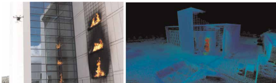
Figure 5. UAV scanning a simulated facade fire on the campus of the Bavarian firefighter school Würzburg (left) and the corresponding 3D model colored by temperature (right). Red indicates high temperatures.
