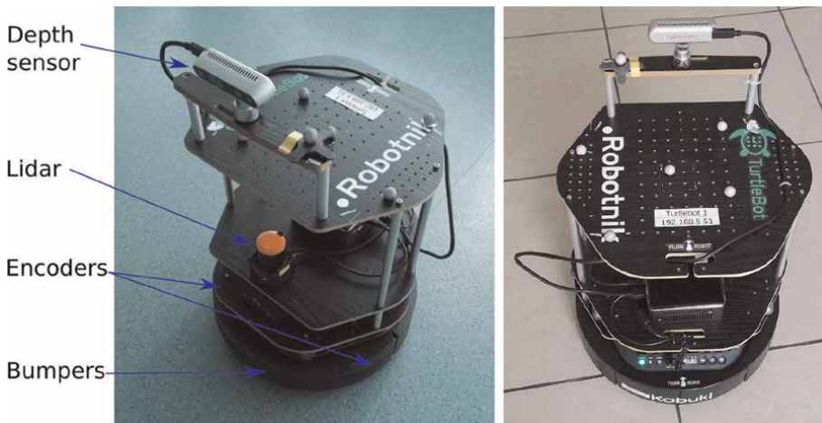
Figure 12. Turtlebot robot equipped with multiple sensors used for localization and mapping.
