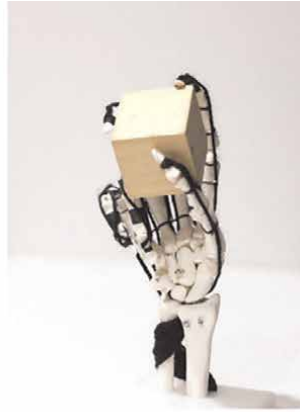
Tripod grasp \varphi = [\varphi_1 \varphi_2 \varphi_3 \varphi_4^{max} \varphi_5^{max} \varphi_6 \ 1]^T
