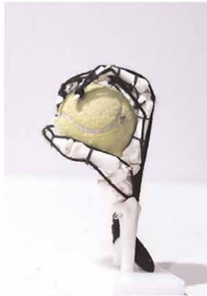
Power grasp sphere (3 Finger) grasp \varphi = [\varphi_1 \varphi_2 \varphi_3 \varphi_4^{max} \varphi_5^{max} \varphi_6 \ 0]^T
