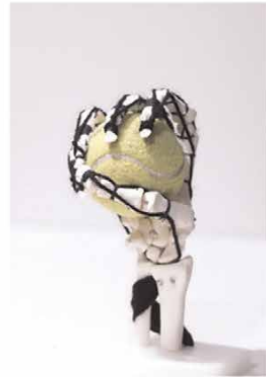
Power sphere grasp \varphi = [\varphi_1 \varphi_2 \varphi_3 \varphi_4 \varphi_5 \varphi_6 \ 0]^T
