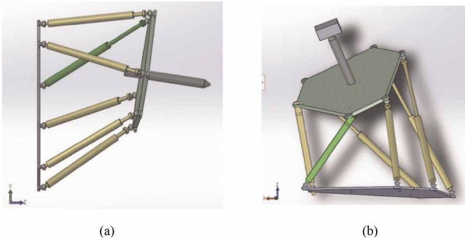
Figure 11. Assessment of kinematics using Solidworks. (a) forward kinematics (b) inverse kinematics.
