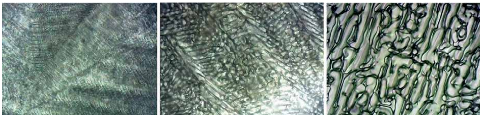
Figure 1. The structure of ice in a 10% \text{Me}_2\text{SO} saline solution in a cryomicroscope at 10x magnification after controlled cooling at different rates to -100^{\circ}\text{C} . samples were cooled, left to right, at 10^{\circ}\text{C}/\text{min} , 1^{\circ}\text{C}/\text{min} and 0.1^{\circ}\text{C}/\text{min} . The extremely low cooling rate used in C results in a markedly different ice structure.
