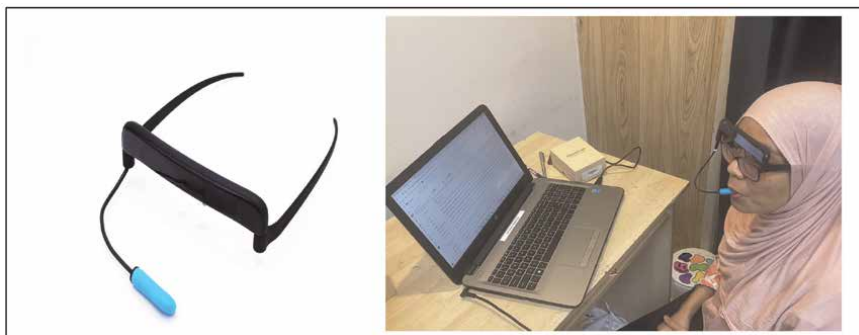
Figure 2. GlassOuse is worn like a pair of glasses and connects to mobile phones, computers, tablets, and smart TVs via Bluetooth. The user moves her head from side to side to navigate the cursor on the screen and bites on the Bite Switch (in cyan) to click items on the computer similar to a computer mouse. (Photo by Intan Sabrina).
