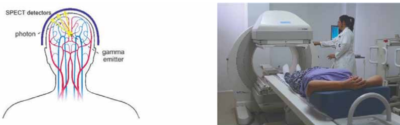
Figure 2. SPECT device uses gamma-emitter radiotracers, which can be given by injection, inhalation, or orally. The SPECT detectors receive the gamma radiation and deliver the signal to the image processing and reconstruction unit [11]. The image on the right is courtesy of IAEA Imagebank.
