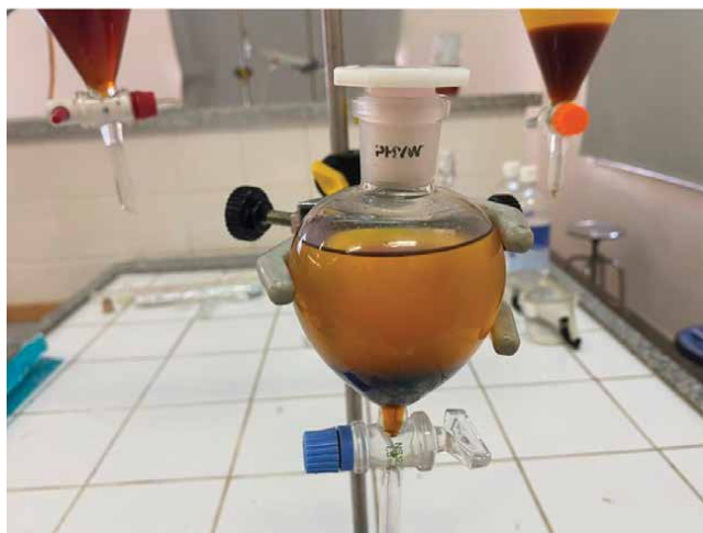
Figure 3. Decanting funnel installed at the bottom of the RD column.
