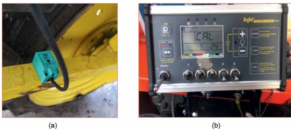
Figure 10. A view of (a) proximity sensor installed at rear wheel and (b) calibration step screen on electronic control unit.
