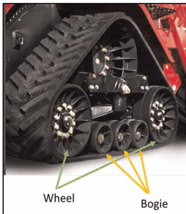
Figure 13. Bogie wheel track design (Case IH, 2022) – [28].
