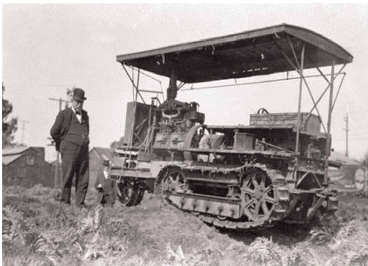
Figure 8. Benjamin Holt testing the first prototype gasoline-powered track-type tractor in 1908 (Caterpillar, Inc., 2021) – [27].
