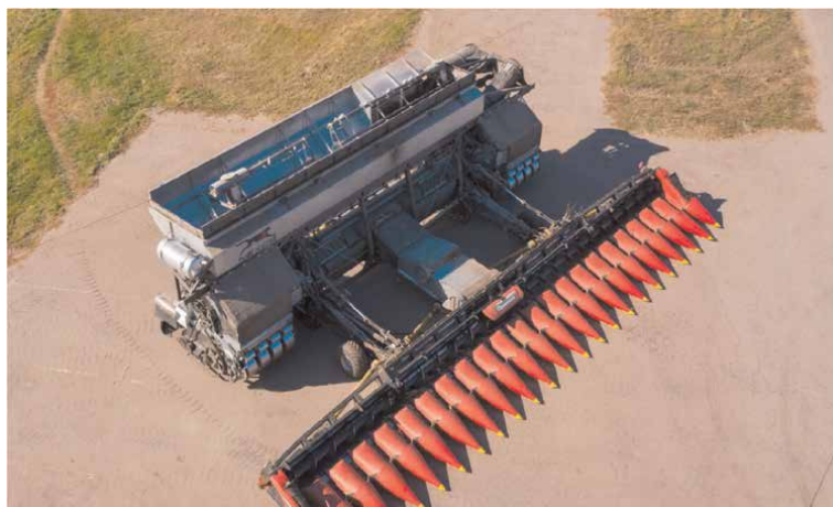
Figure 30. NEXAT system for controlled traffic farming (Misser Uitgeverij B.V., 2021) – [47].
