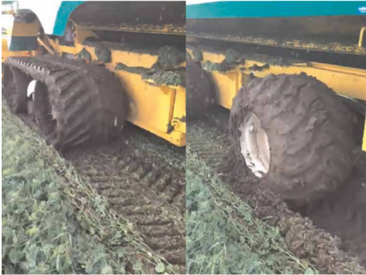
Figure 17. Rut comparison of tracks vs. tires in muddy conditions (Elmers manufacturing Inc., 2019) – [30].
