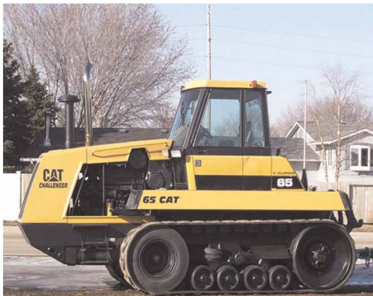
Figure 9. A 1986 Caterpillar challenger 65 ® rubber-tracked tractor (TractorData.com, 2016) – [3].
