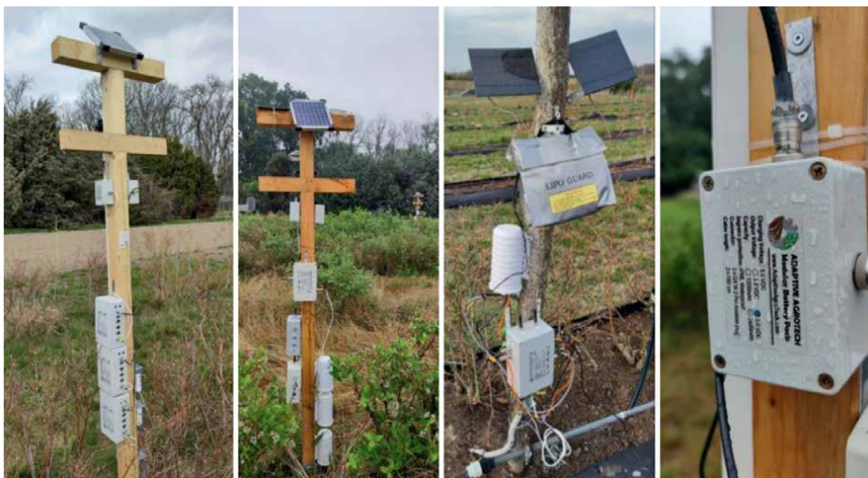
Figure 13. Implementation of multiple solar-powered LoRa sensors in different berry orchards for IoT monitoring of field parameters. Source: SunBot.de.
