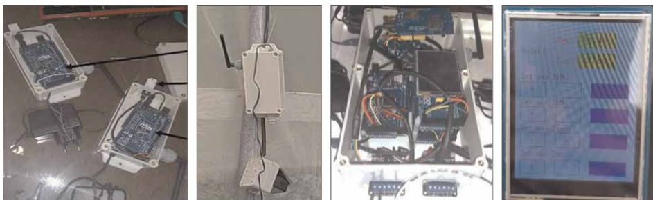
Figure 8. An prototype automation system for small-scale greenhouses [31].
