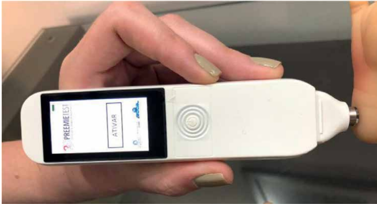
Figure 2. The application of the multiband photometer for predict gestational age prediction in simulated newborn-doll application. Source: The authors.
