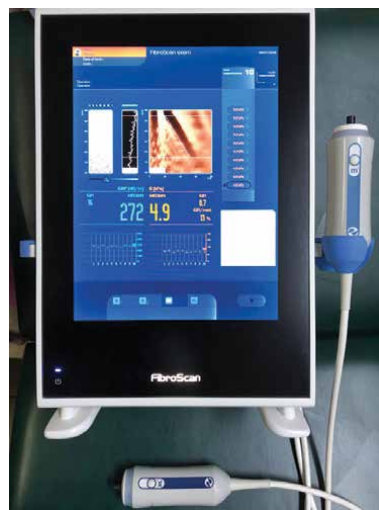
Figure 3. FibroScan (Echosens, Paris, France) with M and XL probes (in light blue CAP values are shown, while in yellow the liver stiffness values).
