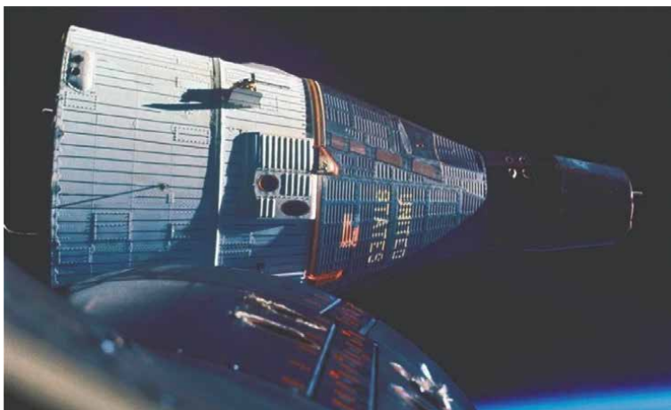
Figure 3. The Gemini spacecraft with the centered, white-painted portion in magnesium alloy.
