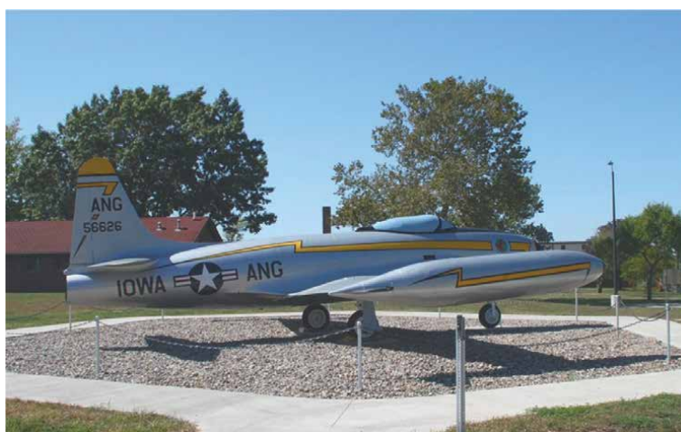
Figure 2. The Lockheed F-80C is constructed of magnesium throughout, today visible at the United States Air Force Museum, Ohio.
