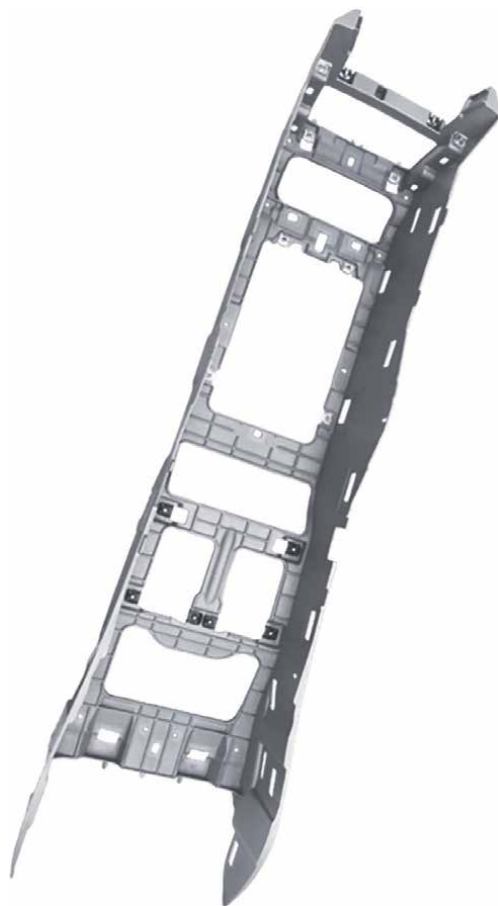
Figure 14. Magnesium AM 50 die cast front center console for Audi A8, high stiffness, no machining and all connection and fixing points are intergrated (courtesy of GF Casting Solutions).
