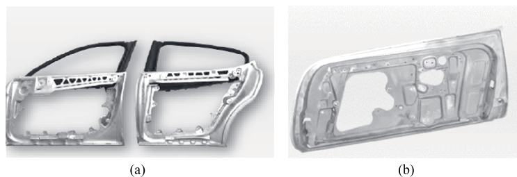
Figure 13. (a) The Porsche window frame realized by AM50 magnesium alloy with multi process stages (casting, laser cutting, machining), finally coated and joined; (b) The Aston Martin cover door made AM50 with multi-stage process (Casting, Stamping, Flattening) [courtesy of GF Casting Solutions AG].
