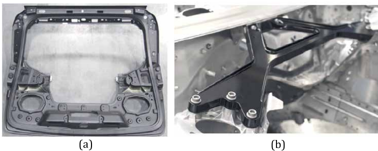
Figure 10. (a) Diecast liftgate inner by Meridien (courtesy of IMA), 1450 mm wide, 1210 mm in height, the mass of 6.9 kg, (b) Strut bar Audi A8 (courtesy of IMA).
