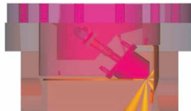
(c) Installation of the multi-hole nozzle
