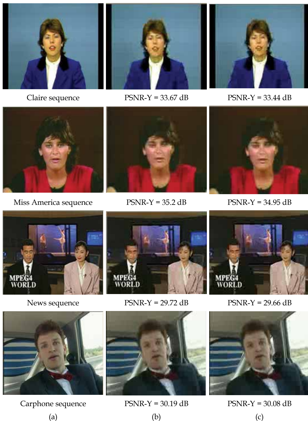
Fig. 23. (a) Original, (b) Reconstructed from SW and (c) Reconstructed from HW/SW of the 12 th frame of the test video sequences
