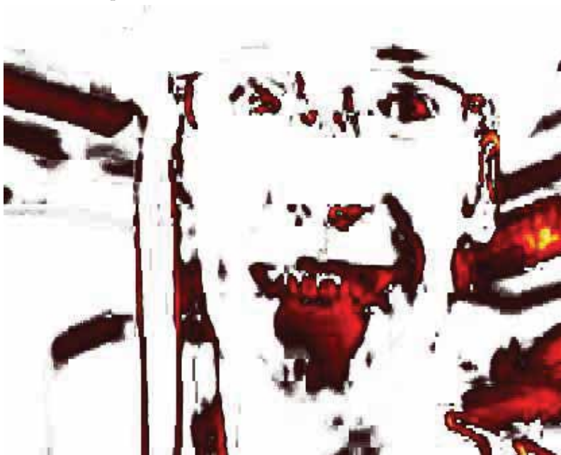
Fig. 3. Variance for the individual pixels in a video sequence. White = low variance Yellow = high variance
