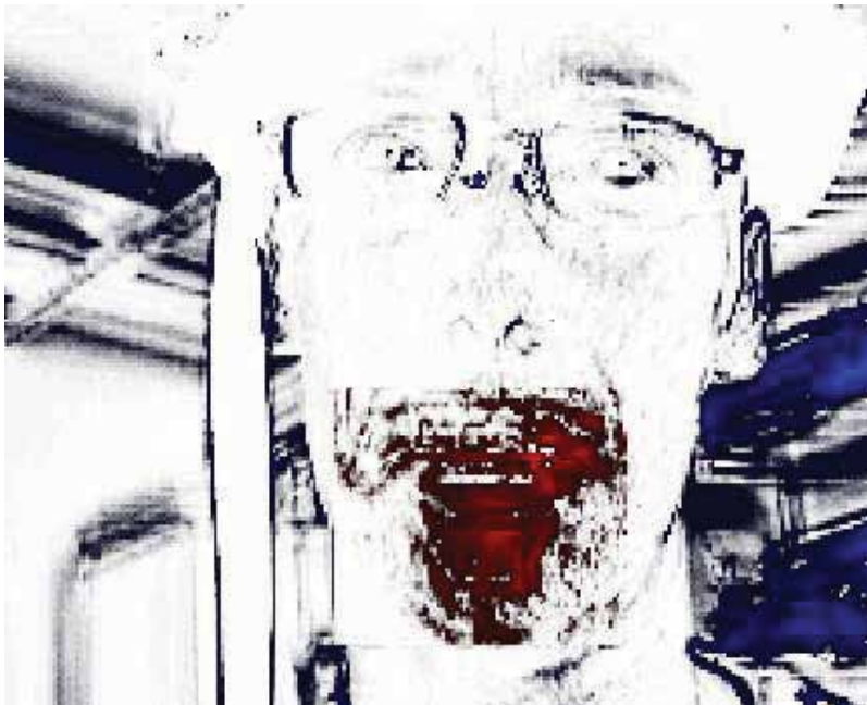
Fig. 4. Individual pixel PSNR for encoding with foreground I^f compared to encoding with the entire frame I red =improved PSNR blue =reduced PSNR.
