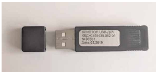
Figure 6. View of random number generator Crypton USB-DRN .
