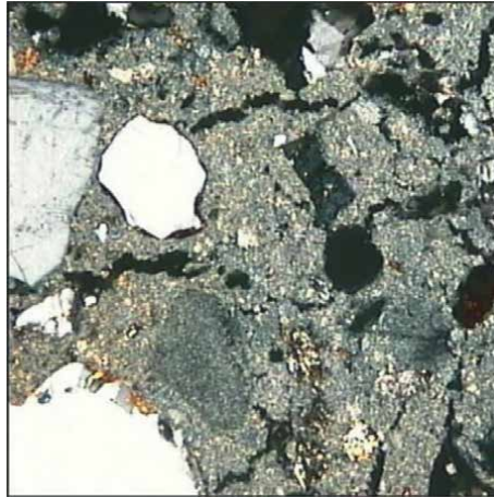
Figure 8. Pores and cracks in the structure of lime mortar with coarse aggregates (polarized microscope, x15).
