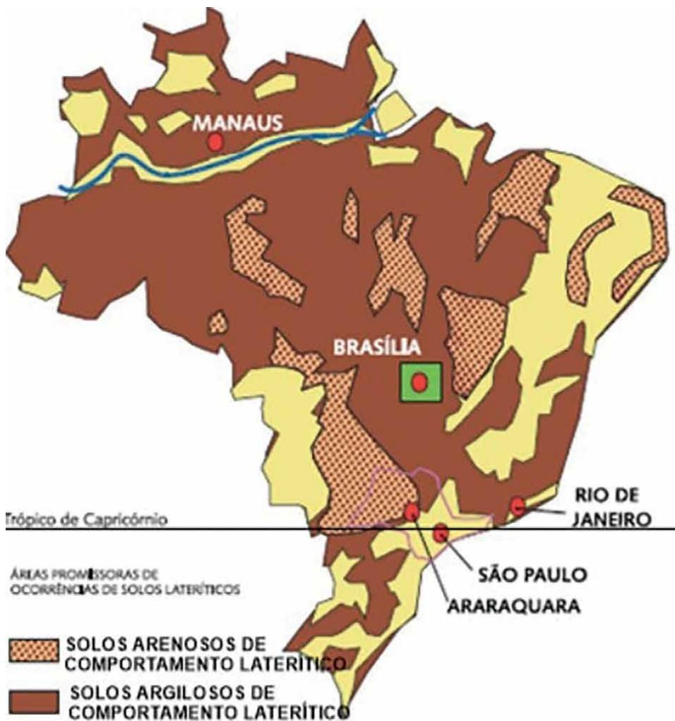
Figure 5. Area of occurrence of laterite soils in Brazil represented by dark brown colors and hachuras [32].
