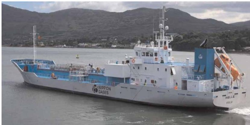
Figure 26. LNG Tanker ships for CO 2 Delivery Offshore EOR projects (OTC 21984).
