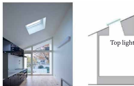
Figure 8. Example of top light utilization in a building.
