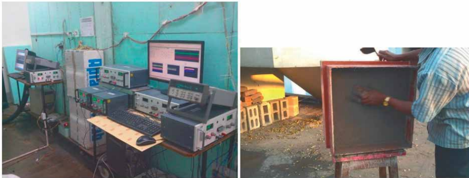
Figure 7. Guarded hot box test setup with data logging and wall panel under preparation.
