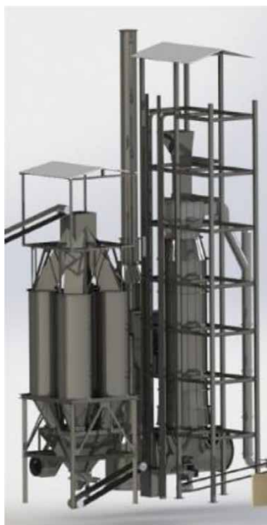
Figure 4. GCS' pyrolysis process with integrated heat capture and utilization.
