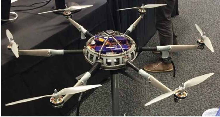
Figure 4. 3D-printed titanium firefighting drone [23].
