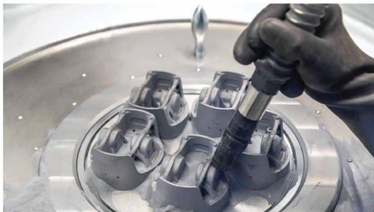
Figure 8. Pistons of the twin-turbo boxer engine of 911GT2 RS [Source: Porsche AG].
