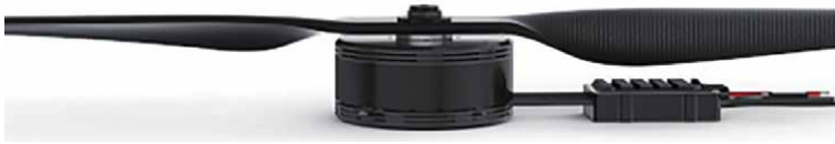
Figure 8. Electric propulsion unit of multirotor type of UAV [31].
