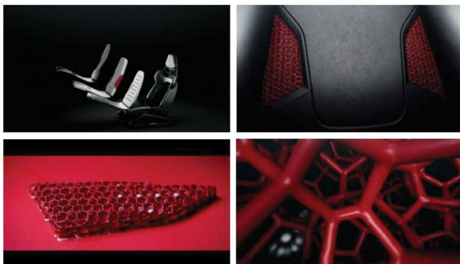
Figure 9. 3D-Printed bodyform full-bucket sports seats [Source: Porsche AG].
