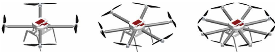
Figure 1. Conventional multirotor UAV configurations in \times -layout.
