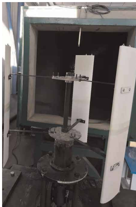
Figure 4. Model of vertical axis wind turbine in wind tunnel test.
