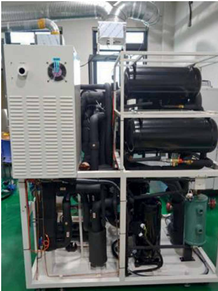
Figure 10. Experimental device of cascade MR refrigerator.
