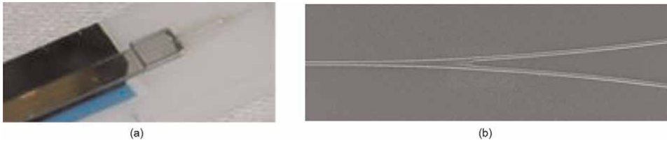
Figure 18. (a) Fibre pig-tailed IO y-branch mounted on mechanical support, (b) SEM picture of the IO Y-junction, allowing beam splitting as well as fibre signal combining.
