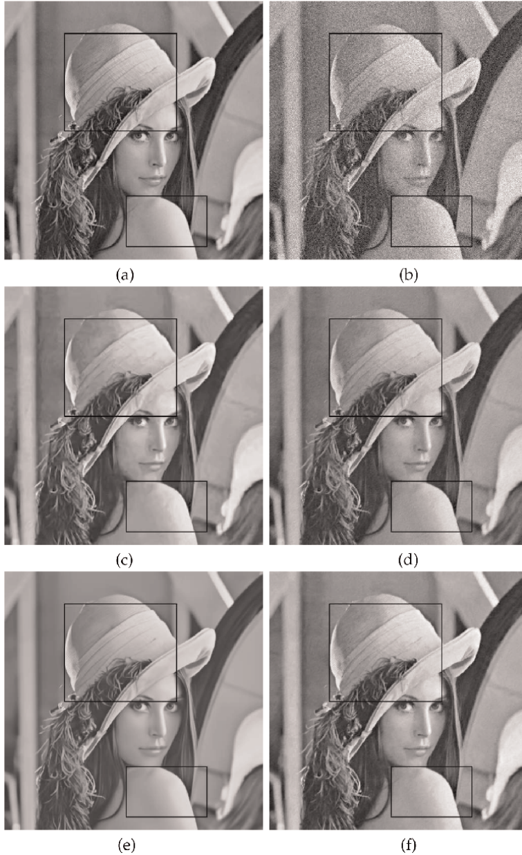
Figure 4. Comparisons of the denoised Lena images derived by BM 3 D, WBN, DRUNet, and graphical ADMM. The noise standard deviation is set at \sigma = 25 : (a) the original 512 \times 512 Lena image; (b) the noised image; (c) the result of BM 3 D; (d) the result of WBN; (e) the result of DRUNet; and (f) the result of graphical ADMM. Graphical ADMM preserves both the smooth and edged areas in the original image, as shown in the highlighted areas.
