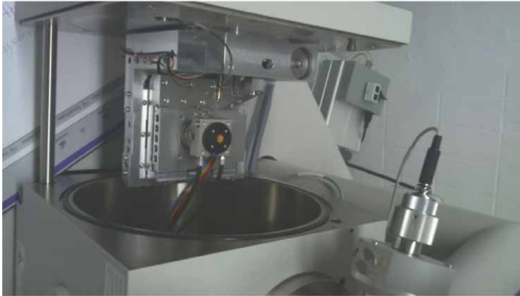
Figure 3. ESEM chamber: Cooling table with circulation cooler, P. Körber.
