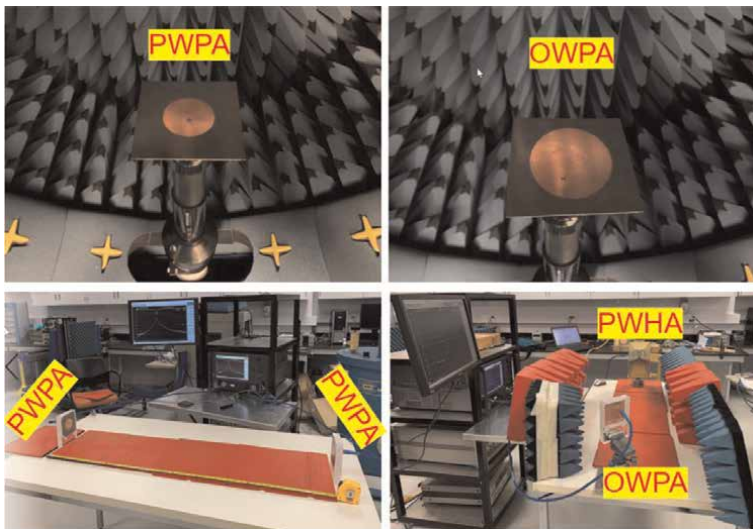
Figure 22. Measurement setup in SATIMO lab and for Tx–Rx configuration.
