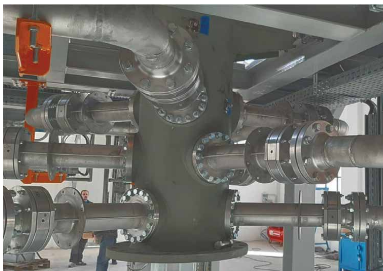
Figure 8. MW oven located in the bottom part of the prototype with, in front, the microwave guide.
