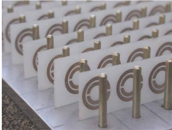
Figure 2. The array of split-ring resonators plus wire assemblies.
