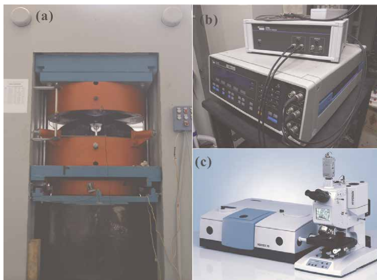
Figure 2. High-pressure conductivity measurement platform and experimental setup in the YJ-3000 t multi-anvil press is equipped in the Key Laboratory of High-temperature and High-pressure Study of the Earth's interior (HTHPSEI), Institute of Geochemistry, Chinese Academy of Sciences, the People's Republic of China. (a) The YJ-3000 t multi-anvil apparatus; (b) the Solartron-1260 and Solarton-1296 interface impedance spectroscopy analyzer operating in the two-electrodes configuration for complex EIS measurements in the frequency range 10^{-4} Hz– 10^7 Hz; (c) the vertex-70v vacuum Fourier-transform infrared spectroscopy (FT-IR) analyzer to check the water content of sample.
