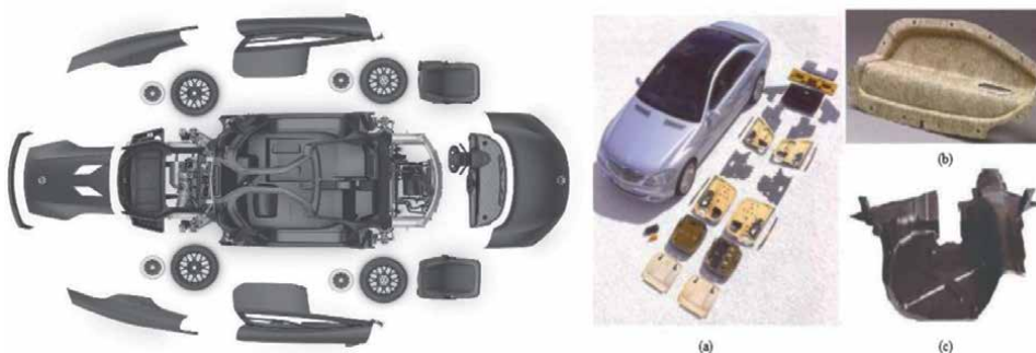
Figure 5. Volkswagen x11 carbon fiber body pieces, adapted from [36] under a creative commons license. (a) the 45 kg of natural fibers in a Mercedes S-class. (b) Car door panel made of natural fibers. (c) Spare wheel cover made of natural fibers.
