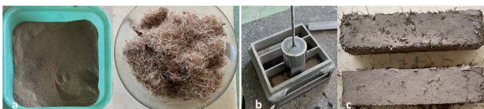
Figure 18. Adobe bricks manufacturing, (a) dry sediment and fibers, (b) miniature proctor for prismatic sample, and (c) molded crude bricks.
