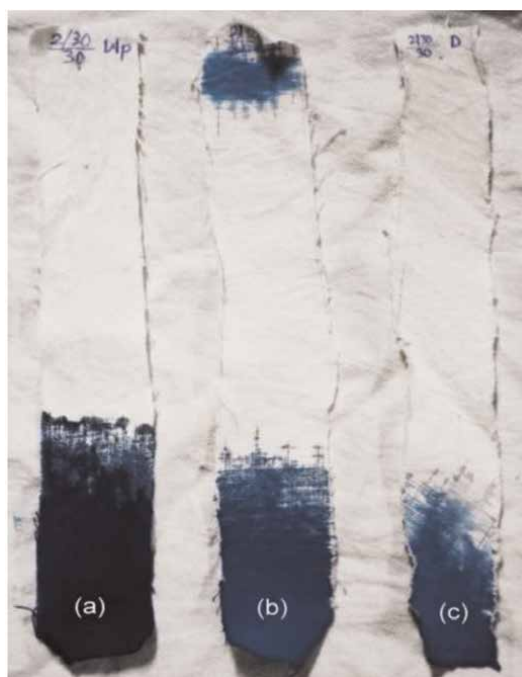
Figure 5. Wicking phenomena in fabric for various directions such as (a) warp way, (b) weft way and (c) diagonal way.
