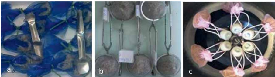
Figure 9. Fabric bags and clips (a) for plant aggregates, tea baskets (b) for plant fibers, fiber bags (c) for centrifugal spinning and Wa ranges for different fibers [20, 25].
