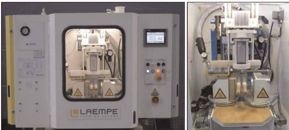
Figure 5. Laempe L1—1-liter core blower.
