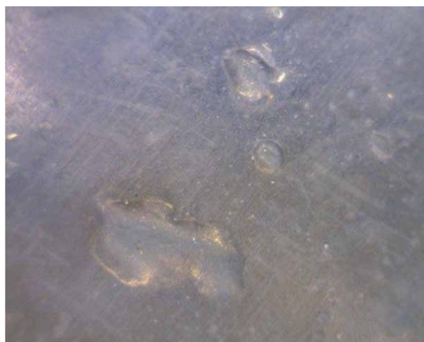
Figure 12. Image of blistering on metal [23].
