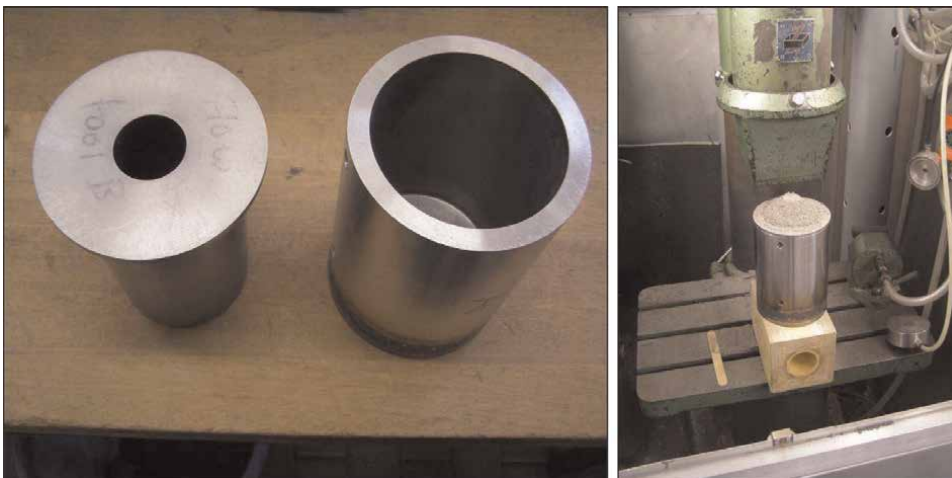
Figure 13. Special type of core box for flowability measurements.
