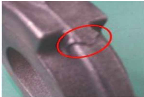
Figure 13. Image of cold lapping of a metal represented below [24].
