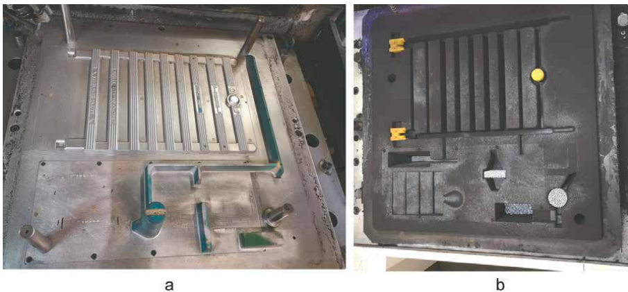
Figure 7. Model plate and mould for research on the production of VM cast iron using the Inmold technology on the FBO line; a/ upper model plate, b/ lower mould [9].
