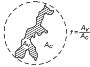
Figure 9. Scheme of shapes of graphite precipitates cross sections [10].
