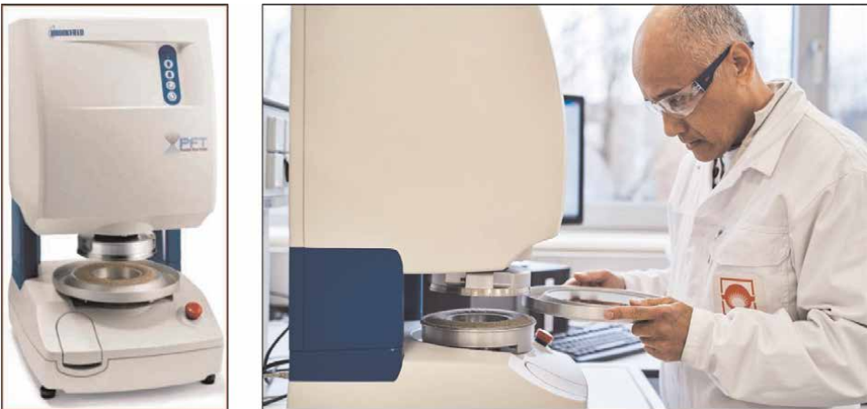
Figure 3. PFT powder flow tester to measure flowability of powders and sand mixtures.
