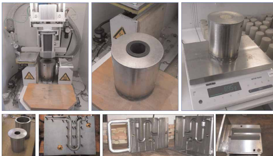
Figure 4. Various types of core boxes with different complexities to measure flowability of different sand mixture compositions.
