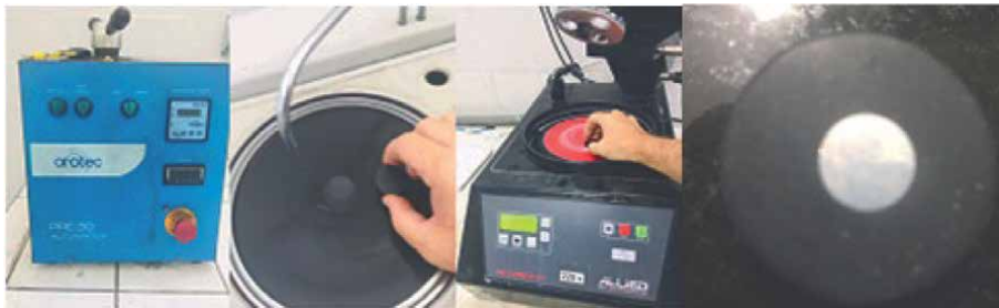
Figure 9. Mounting, sanding, polishing, and finished sample.
