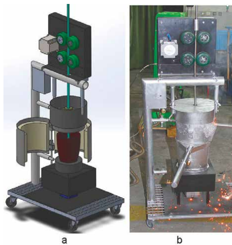
Figure 5. Experimental stand for cast iron nodularisation with the PE method): a/ drawing; b/ processes performed by cored wire method – Precision dispensing Mg.
