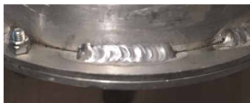
Figure 5. GTAW/TIG fillet weld on aluminum material.
