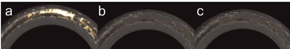
Figure 6. Different filters applied on a sector of the same injector contour image. (a) No filter. (b) Median fill filter. (c) Patch filter.
