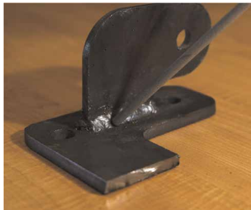
Figure 7. Base material orientation and working location for horizontal position fillet weld (2F).
