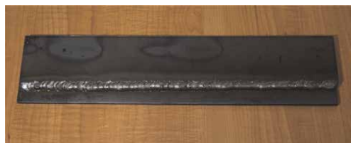
Figure 4. Horizontal fillet weld on clean material done by GMAW/MIG welding.
