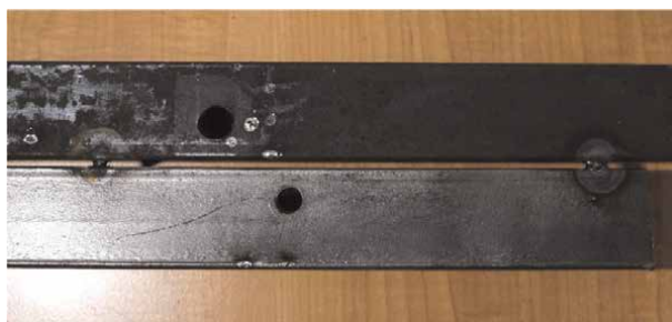
Figure 18. Tack welds applied to establish a 0.3 cm gap between the separated pieces.
