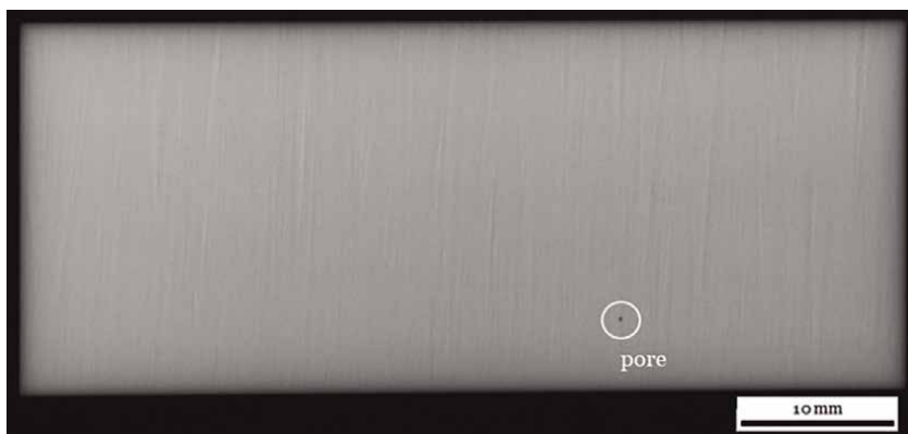
Figure 12. X-ray test on the example of SN 7718 AM wall welded with ArH.
