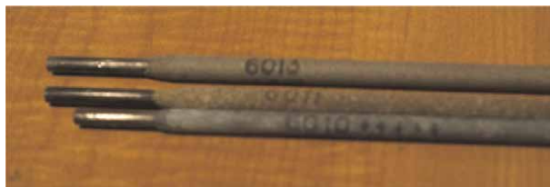
Figure 1. Electrode specification stamped on the flux coating of a typical welding rod.
