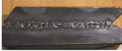
Figure 19. Multiple large tack welds used to fill the gap between the separated pieces, where a continuous weld would likely blow through the gap.
