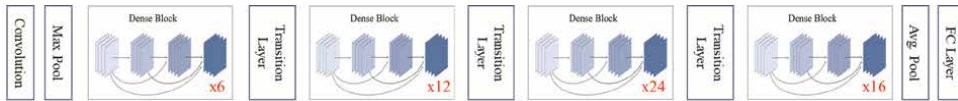
Figure 5. Schematic representation of the layers and blocks in the DenseNet-121 deep learning architecture.
