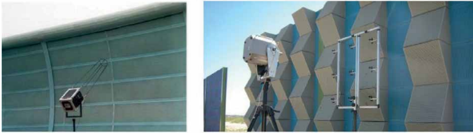
Figure 2. Measurement according to the “Adrienne” method (left) [30] and “QUIESST” method (right) [31].
