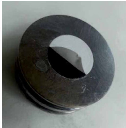
Figure 3. Demonstration of the method used for pressing powdered silica samples onto indium foil [31].
