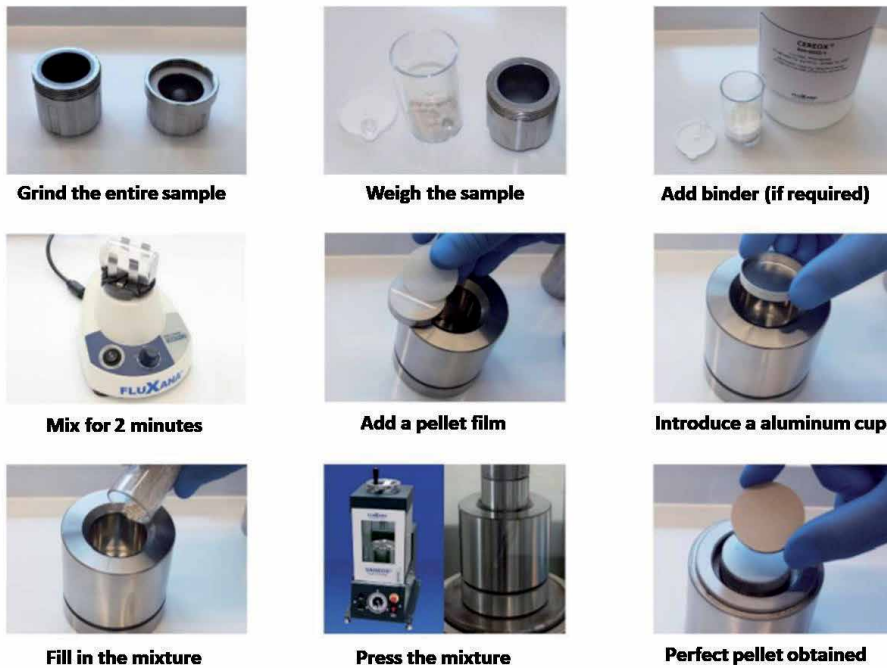
Figure 5. Demonstration of the method used for the preparation of pellets from powdered silica samples [33].
