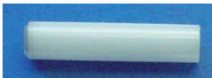
Figure 11. A general torlon based rotor was used for 29 Si solid-state NMR technique [38].
