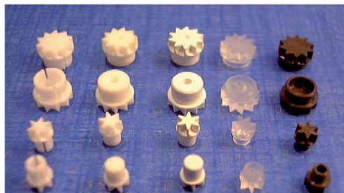
Figure 8. Type of caps used for rotors (typical materials used \text{ZrO}_2 , Macor, KeI and Vespel) [40].
