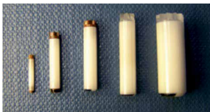
Figure 7. Rotors of different capacities are used for sample packing in ^{29}\text{Si} solid-state NMR [40].
