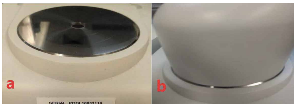
Figure 5. Front view of FTIRS-NIR (a) uncovered diffuse sample port, (b) covered sample port with standardized black reference.
