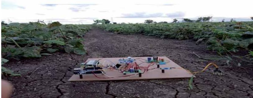
Figure 15. Experimental setup of hardware kit to collect NPK values.
