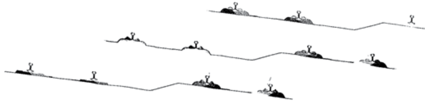
Figure 7. Illustration of transversal profiles of both railway lines obtained by numerical analysis of clouds of data.
