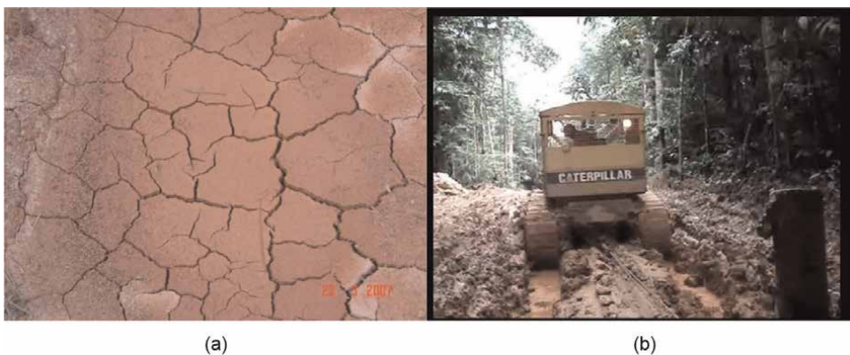
Figure 5. (a) Topsoil after natural drying. (b) Loss of resistance of soil with a dispersed structure (right) (photos: NS Campelo).
