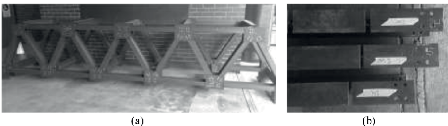
Figure 15. (a) Experimental model of a steel truss bridge and (b) imposed damages [51].
