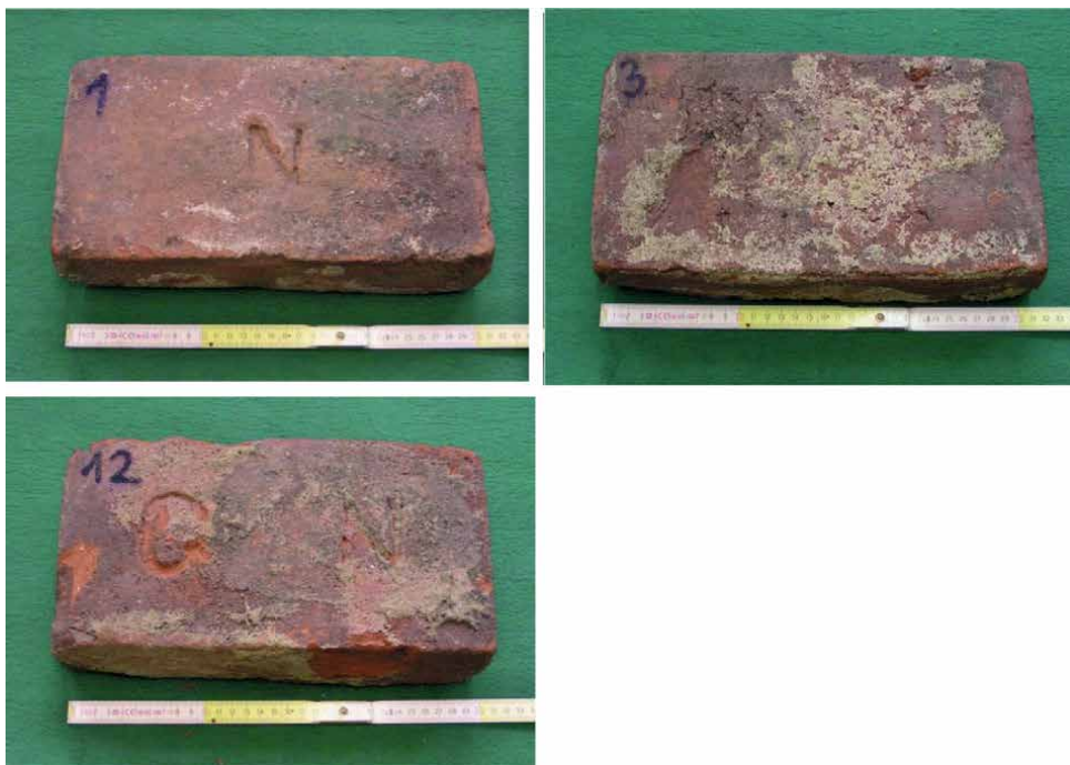
Figure 12. The bricks used for laboratory testing are marked “N” (Nicolzburg). Their appearance and dimensions correspond to early baroque bricks except lower and wider brick N 12 from a later period (marked “GN”) [4].
