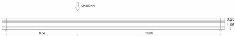
Figure 7. Point load of 300 kN at a distance equivalent to L/3 from one of the supports of a beam.
