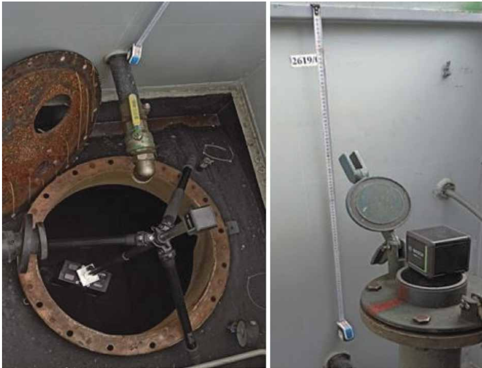
Figure 1. Scanning of the horizontal cylindrical underground tank through its hatch.
