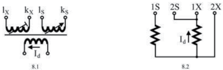
Figure 8. Input sensor elements of means for comparing two secondary currents of the CTs.
