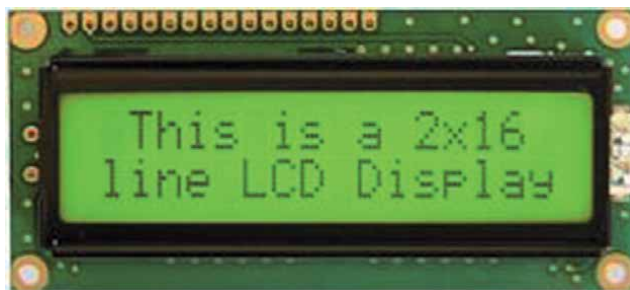
Figure 1. 2 \times 16 LCD physical picture [5].
